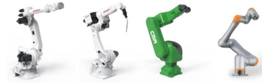
General Industrial Robot      Welding Robot      Painting Robot      Cobot
